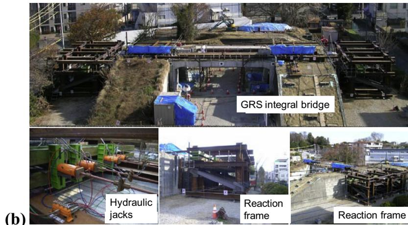
Fig. 13. (a) A full-scale model of GRS integral bridge, completed Feb. 2009 at Railway Technical Research Institute, Japan (Suga et al., 2012); and (b) cyclic lateral loading tests applying simulating thermal deformation of the girder and level 2 design seismic loads (Jan, 2012) Koda et al., 2013.
