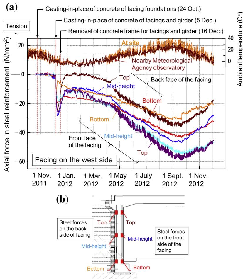
**Fig. 18.** (a) Time histories of ambient temperature and axial forces in the steel reinforcement in the west side facing; and (b) locations of measurement.
