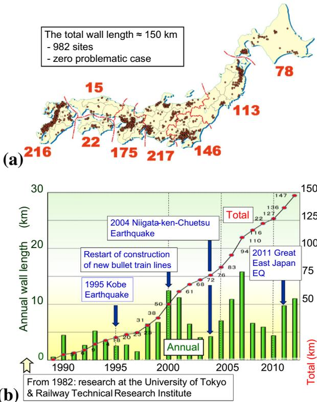
Fig. 7. (a) Locations; and (b) history of GRS RWs with a stage-constructed FHR facing as of June 2013.
