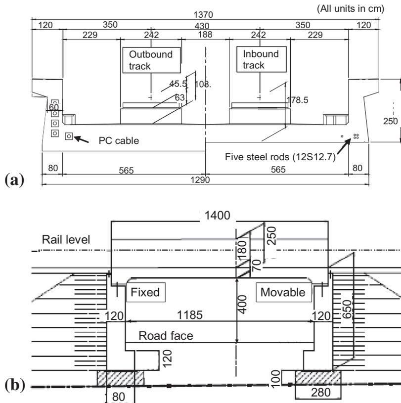
**Fig. 16.** PC through bridge (alternative plan 1): (a) transversal cross-sections of the girder at the top of the facing (left) and the center (right); and (b) longitudinal cross-section of the bridge.
