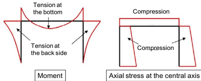
Fig. 19. Schematic diagram showing the stress distribution patterns in the steel reinforcements when subjected to the self-weight of RC members.
