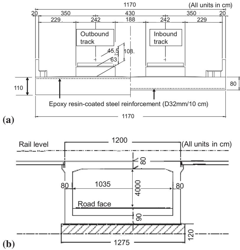
**Fig. 15.** Box culver (the original plan): (a) transversal cross-sections of the girder at the top of the facing (left) and the center (right); and (b) longitudinal cross-section of the bridge.
