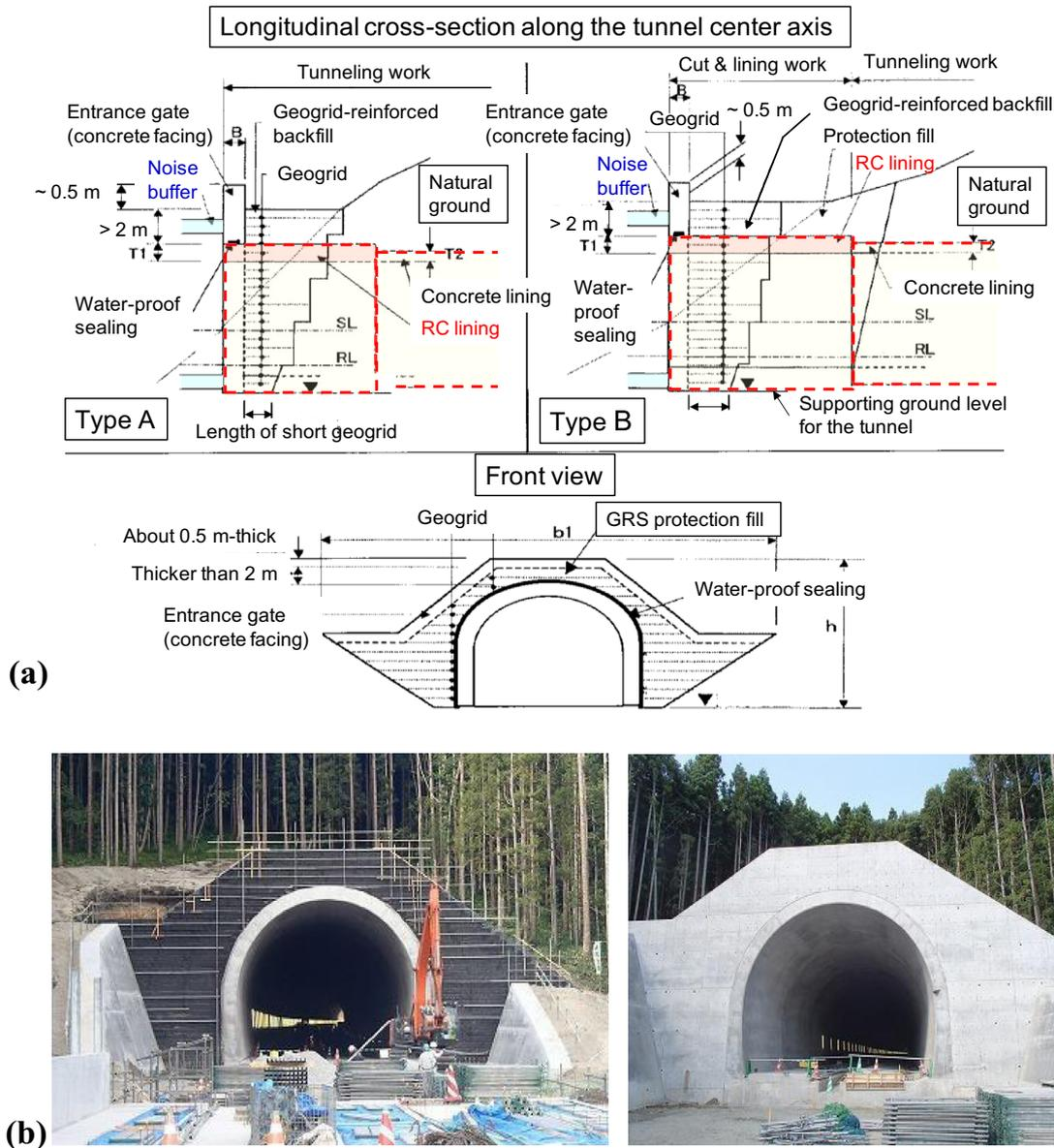
Fig. 23. GRS Tunnel Entrance Protection: (a) two types: and (b) before and after the construction of the front facing at site T10 (at the entrance of Mantaro tunnel).
