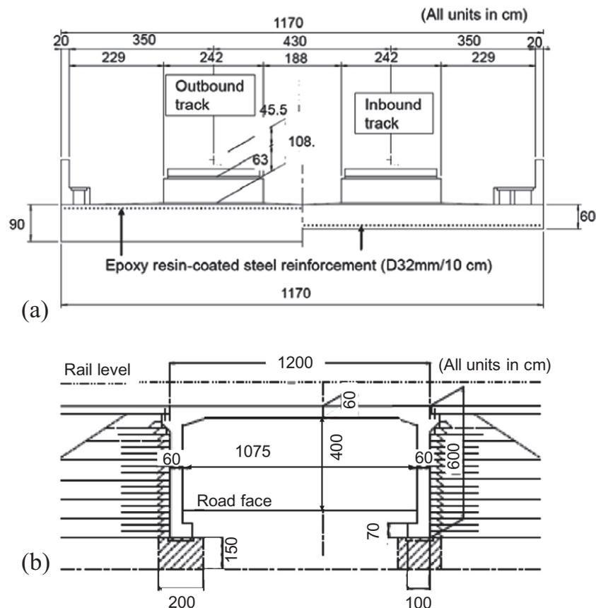
Fig. 17. GRS integral bridge (alternative plan 2): (a) transversal cross-sections of the girder at the top of the facing (left) and the center (right); and (b) longitudinal cross-section of the bridge.
