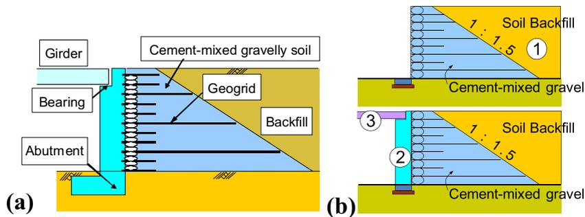
Fig. 10. GRS bridge abutment; (a) structure; and (b) construction procedure.
