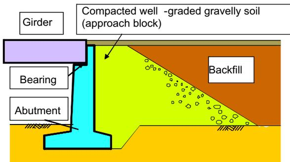
Fig. 9. Improved conventional type bridge abutment having an approach block.
