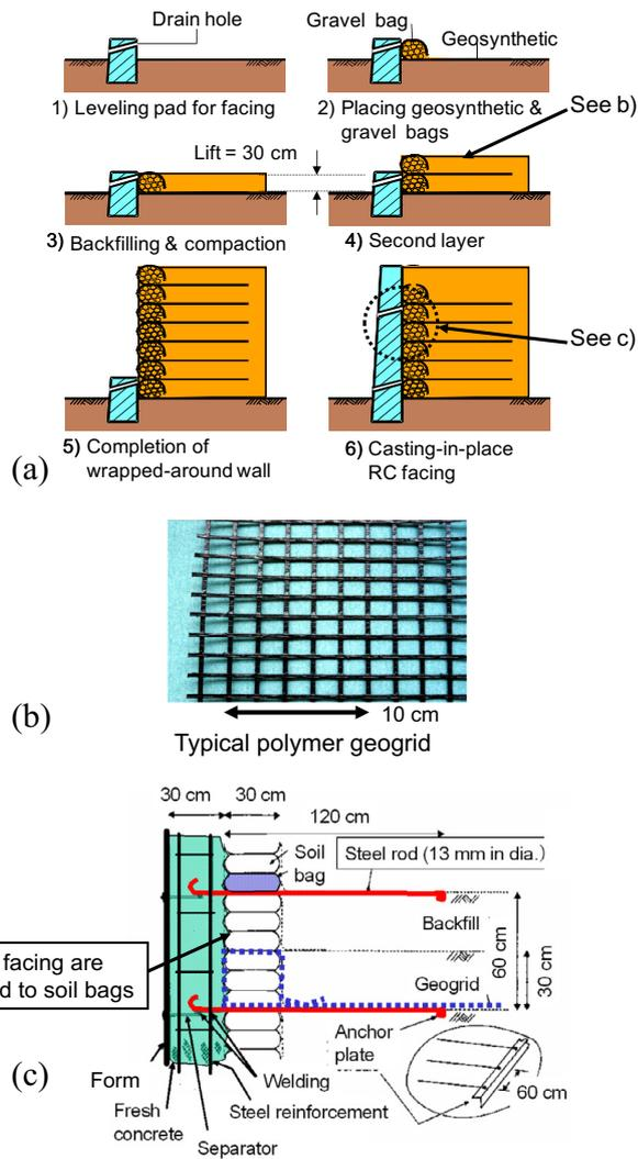
Fig. 3. GRS RW with FHR facing: (a) staged construction; (b) a typical geogrid; and (c) details of facing construction (Tatsuoka et al., 1987).
