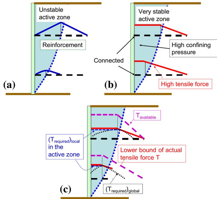
**Fig. 5.** Schematic figures showing effects of firm connection between the reinforcement and the rigid facing on the distribution on tensile forces ( $T$ ) in the reinforcement  $T$  (Tatsuoka, 1992): (a) when the connection force is zero; and (b and c) when connection force is high.
