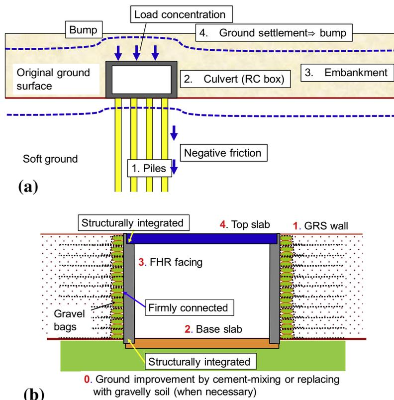
**Fig. 22.** (a) Typical problems with a box culvert structure crossing motorway/railway embankment constructed by the conventional method on a deep soft deposit (the numbers indicate the construction sequence); and (b) most recommendable construction method of a box culvert taking advantage of the “GRS RW with FHR facing technology” (Fig. 3): the numbers show the construction sequence.
