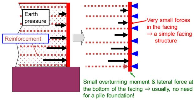
Fig. 6. Mechanical features of FHR facing (Tatsuoka et al., 1987).
