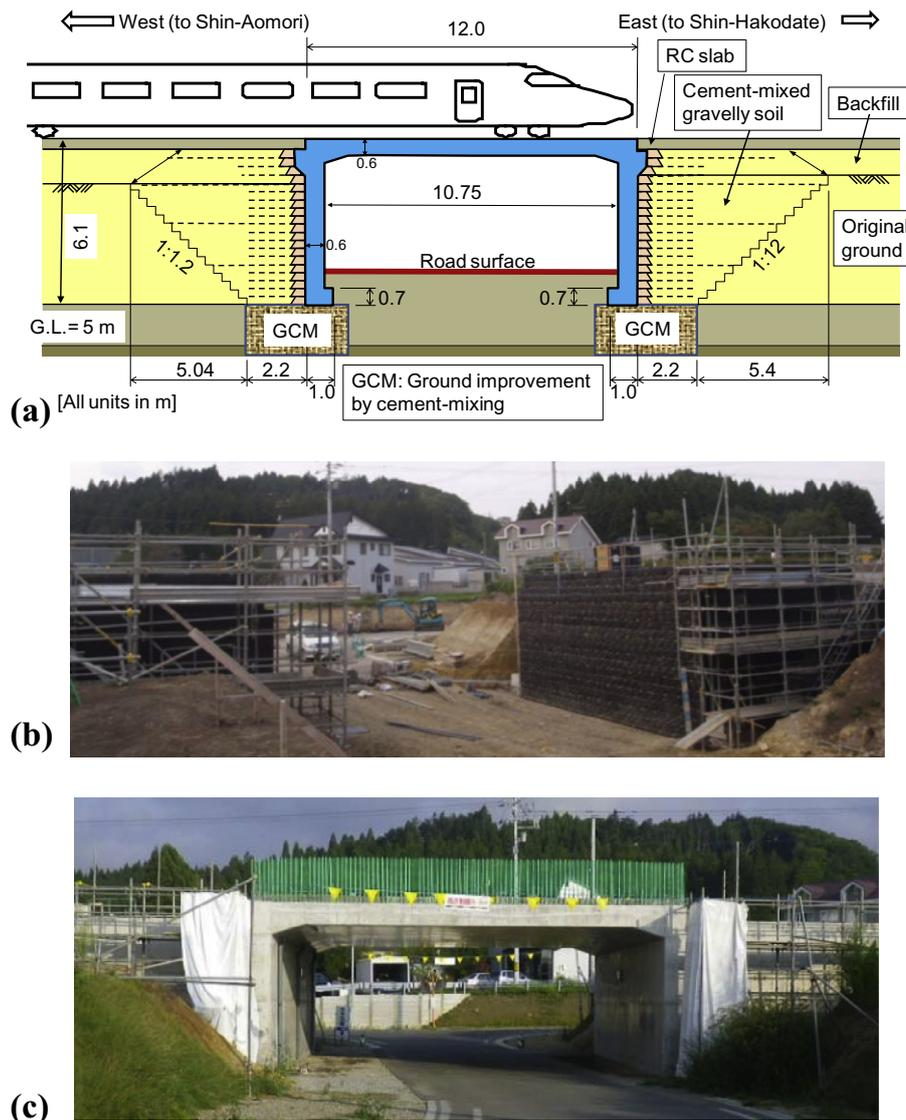
Fig. 14. GRS Integral Bridge at Kikonai (at site I in Fig. 2): (a) structural details; (b) during construction (14 Oct. 2011); and (c) completed (31 July 2012).
