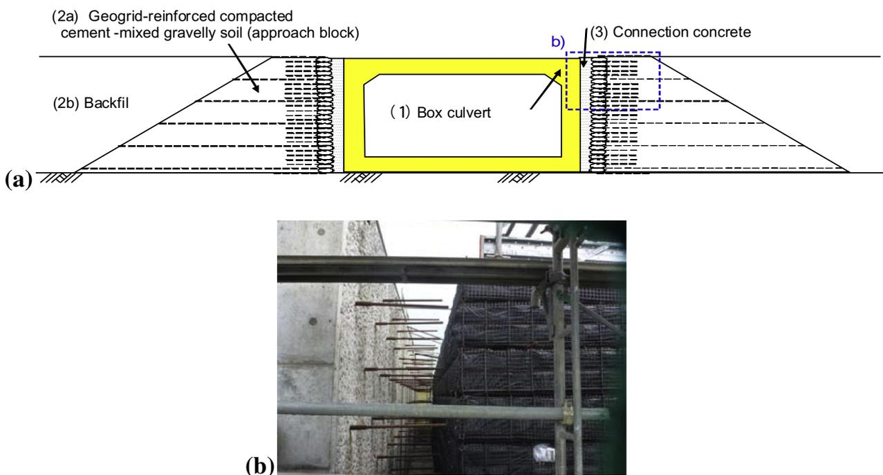
Fig. 20. GRS culvert box (site B2): (a) general structure; the numbers show the construction sequence; and (b) a space between the RC box structure and the approach block before step (3) (at site B1).
