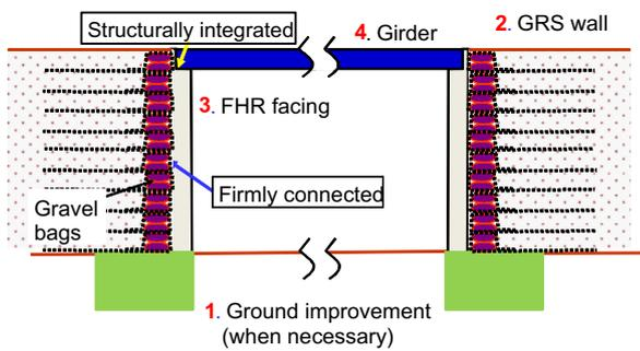
Fig. 12. Structure of GRS integral bridge (the numbers show the construction sequence).
